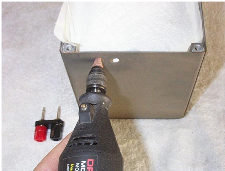
Figure 7.3: Grind Input Jack Holes For A 5-Way Binding Post
