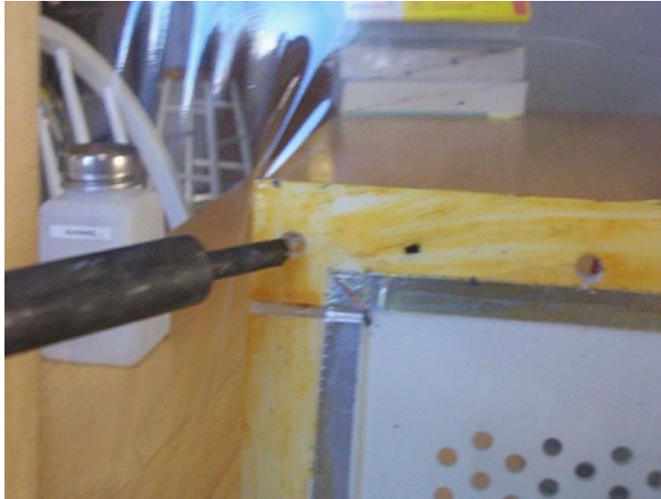
Figure 4.15: Bass Diaphragm Rivet Hole Melting
