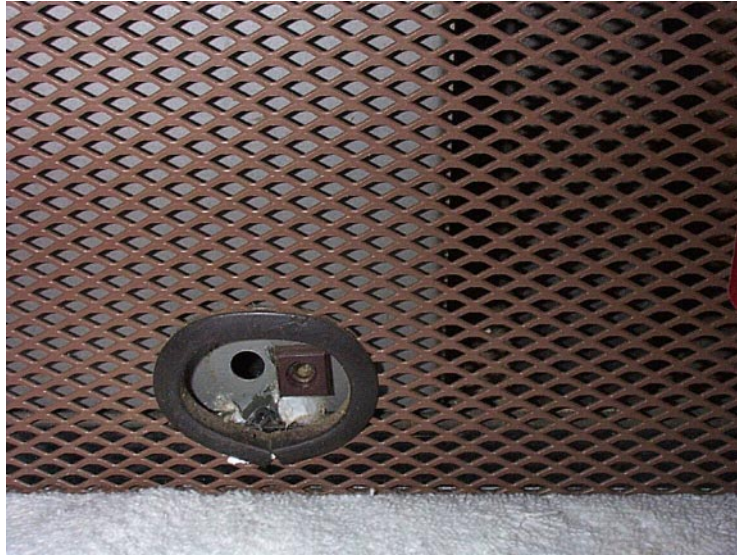
Figure 3.6: Broken Input Banana Connector
