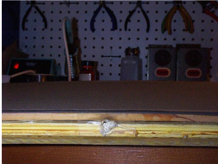
Figure 8.21: Problems Caused By too Long Side Panel Screws
