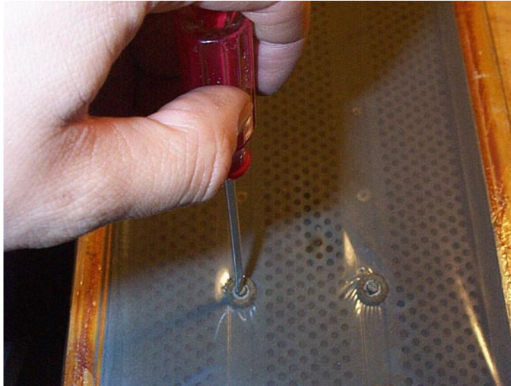
Figure 5.3: Removing The Dust Cover Retaining Screw Assemblies
