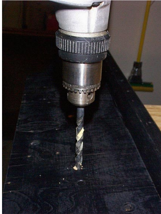
Figure 9.6: Drilling Holes For Stand Hardware
