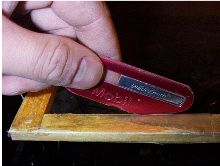
Figure 4.19: Bass Panel Dust Cover Removal
