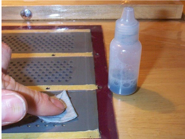
Figure 5.20: Applying ITO Coating To Treble Panel
