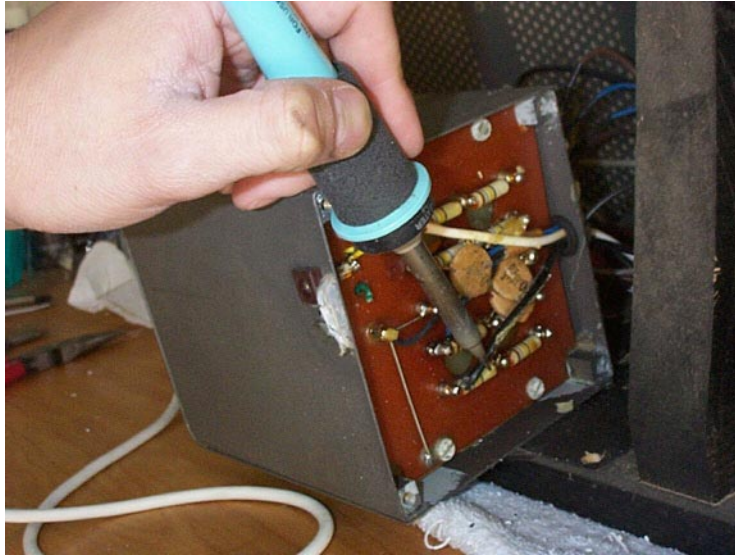
Figure 3.15: Unsolder Input Transformer Connections
