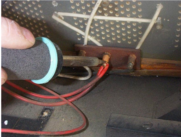
Figure 3.18: Unsolder Bass Panel Connections
