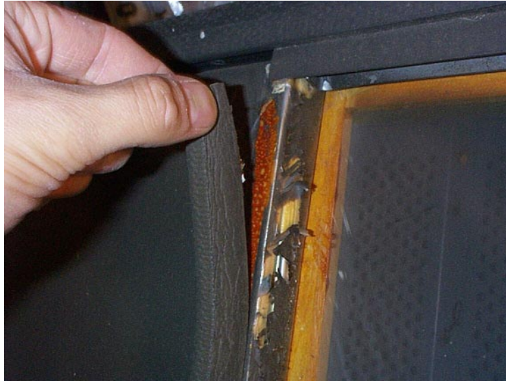
Figure 3.10: Removal of Front Grille Foam Padding
