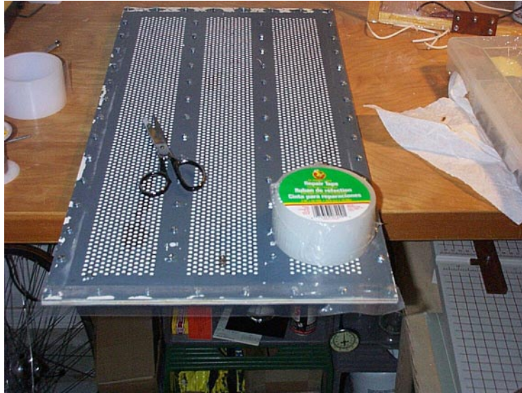
Figure 4.17: Bass Panel Insulating Tape Application
