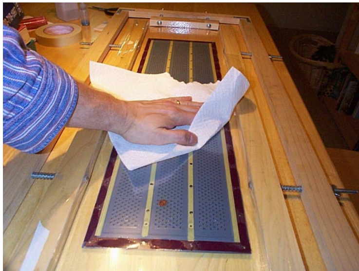
Figure 5.17: Smoothing Treble Panel Epoxy
