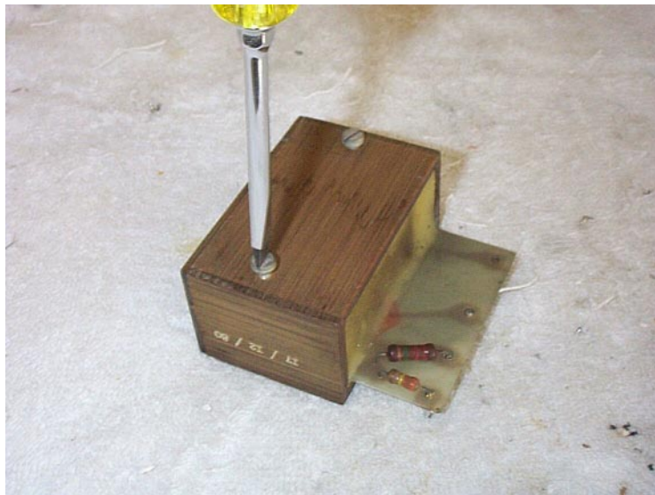
Figure 6.5: Replace EHT Screws
