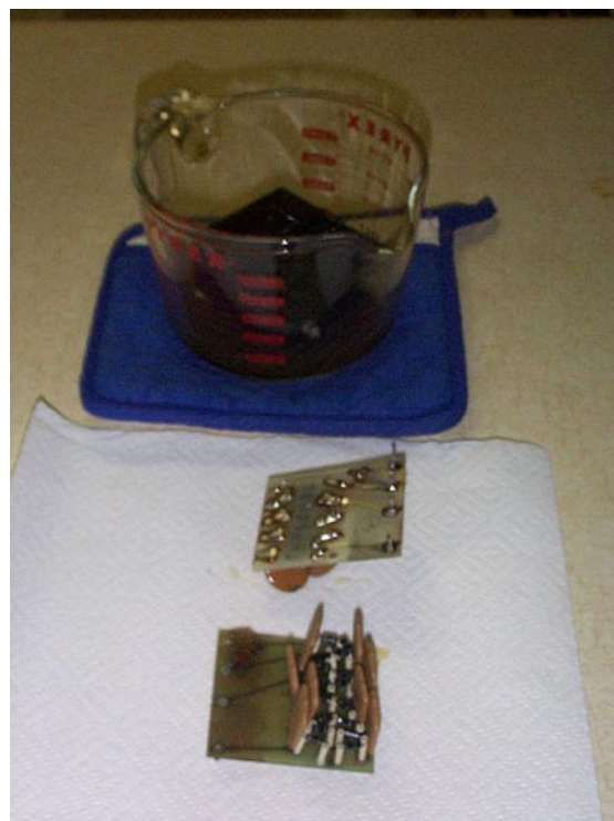
Figure 6.7: EHT Boards Removed From Melted Wax
