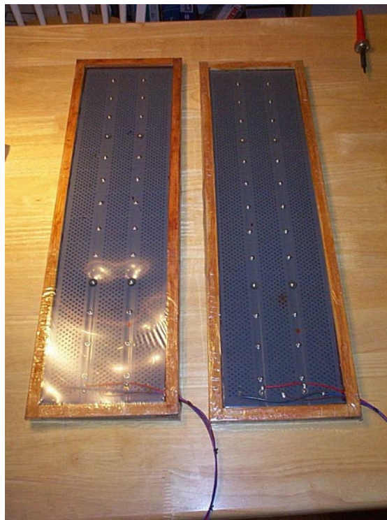
Figure 5.25: Finished Treble Panels
