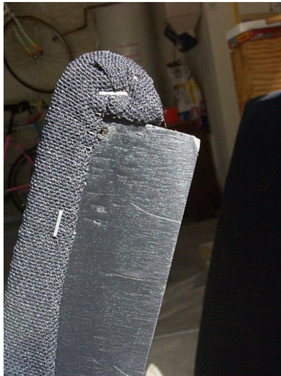
Figure 9.4: Stapling The Grille To the ESL Frame
