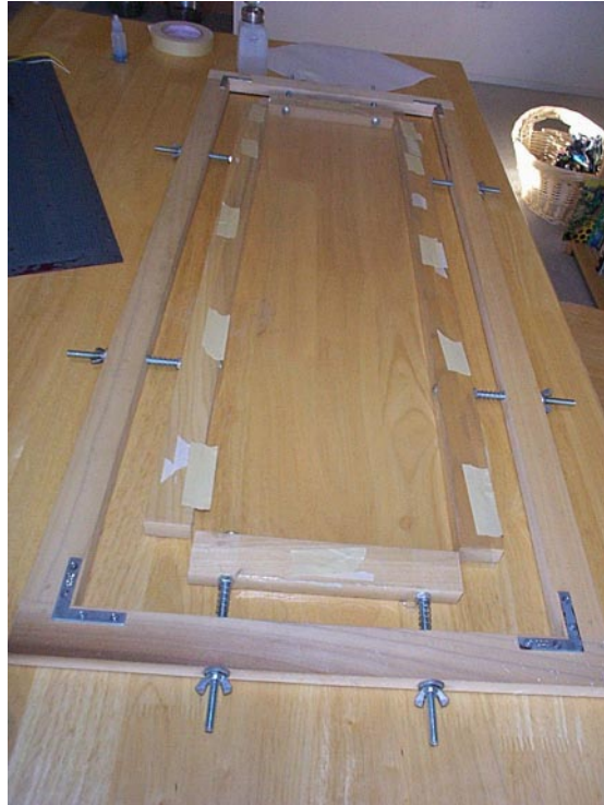
Figure 5.14: Mylar Diaphragm Taped To Stretching Jig
