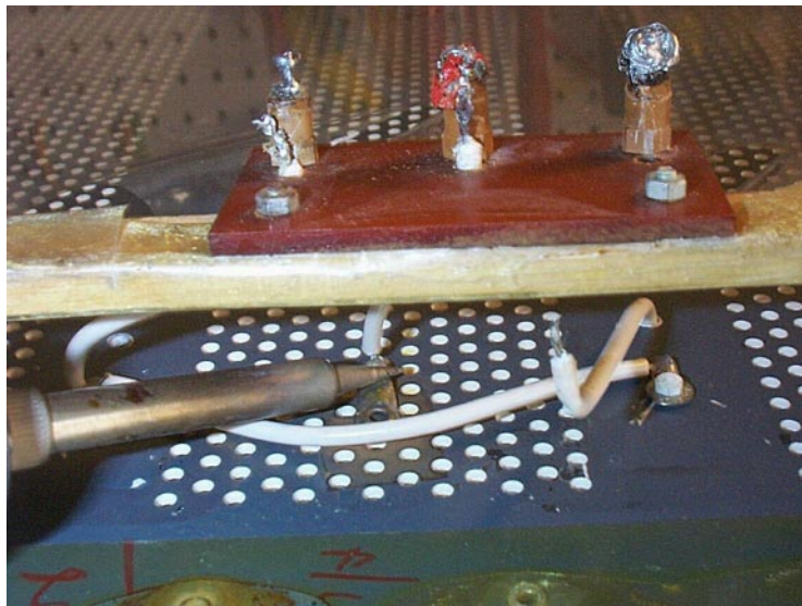
Figure 4.3: Un-soldering Rear Bass Stator Wire
