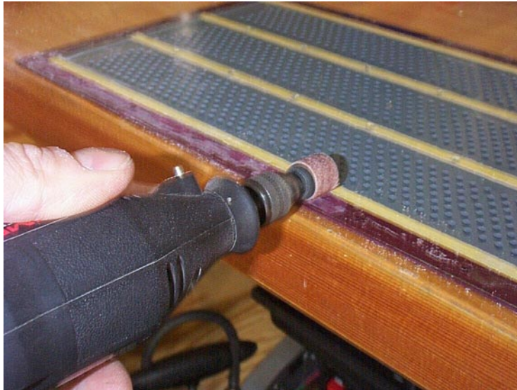
Figure 5.11: Grinding Epoxy On Previously Rebuilt Panel
