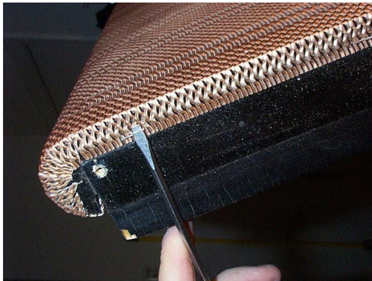
Figure 3.7: Removal of Front Grille Staples
