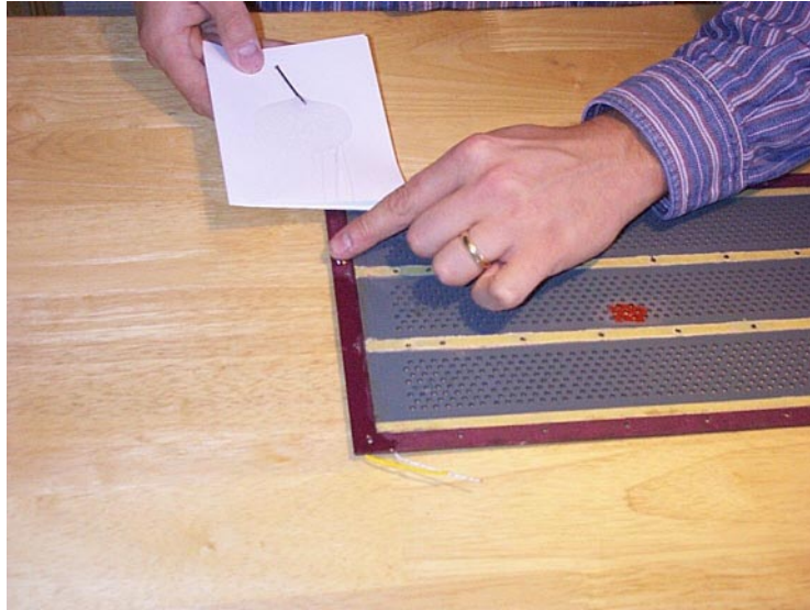
Figure 5.16: Application of Treble Panel Epoxy
