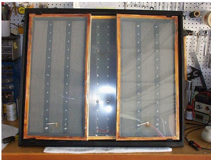
Figure 8.3: Second Bass Panel Installed In Frame
