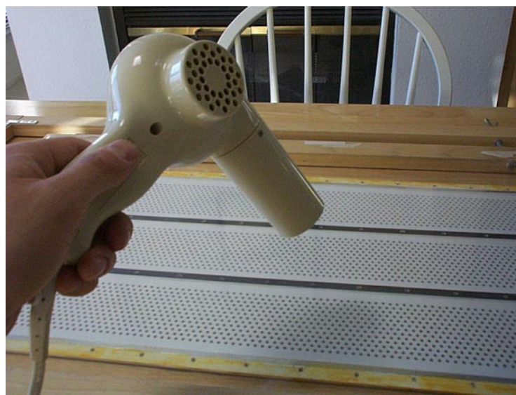
Figure 4.14: Bass Diaphragm Heat Shrinking
