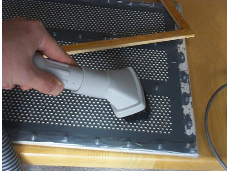
Figure 4.22: Bass Panel Dust Removal
