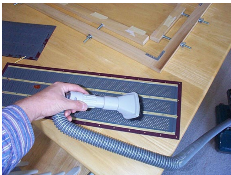
Figure 5.15: Vacuuming Panels And Mylar Diaphragm
