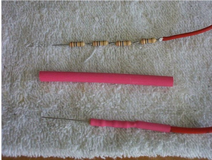
Figure 8.12: Soldering Bias Resistors In Place
