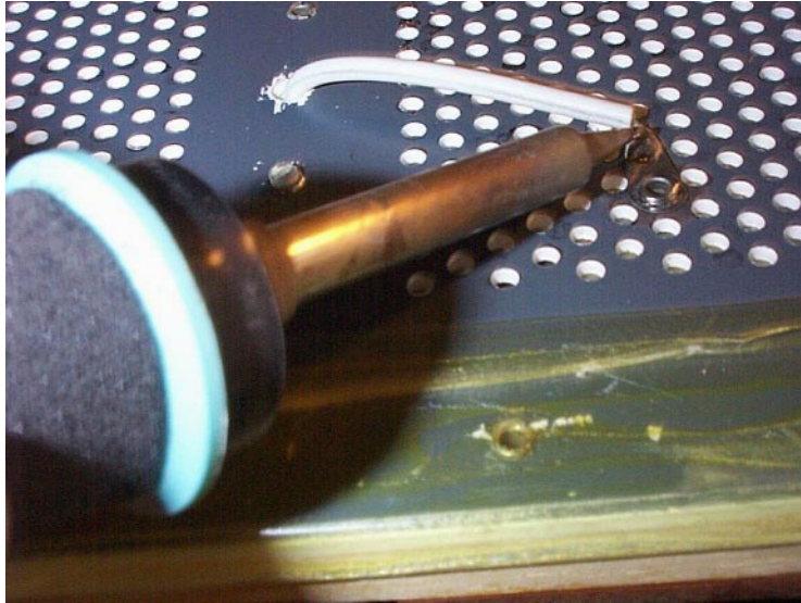
Figure 4.4: Un-soldering Front Bass Stator Wire
