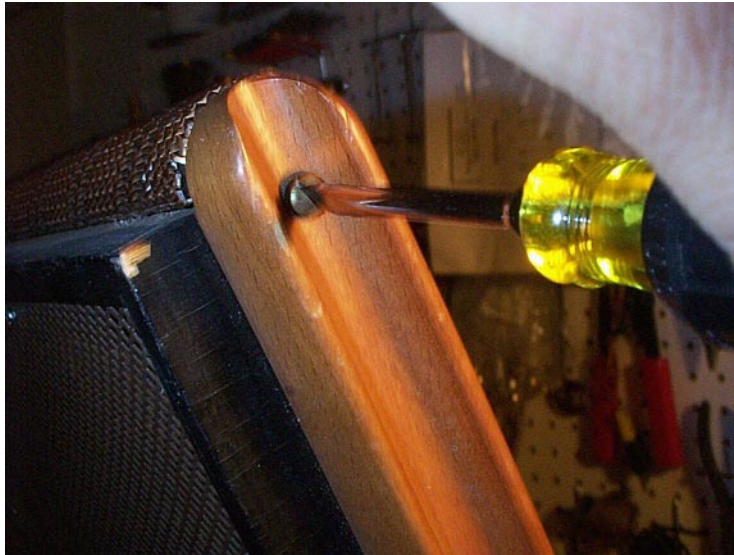
Figure 3.1: Removal of Wooden Trim Strips
