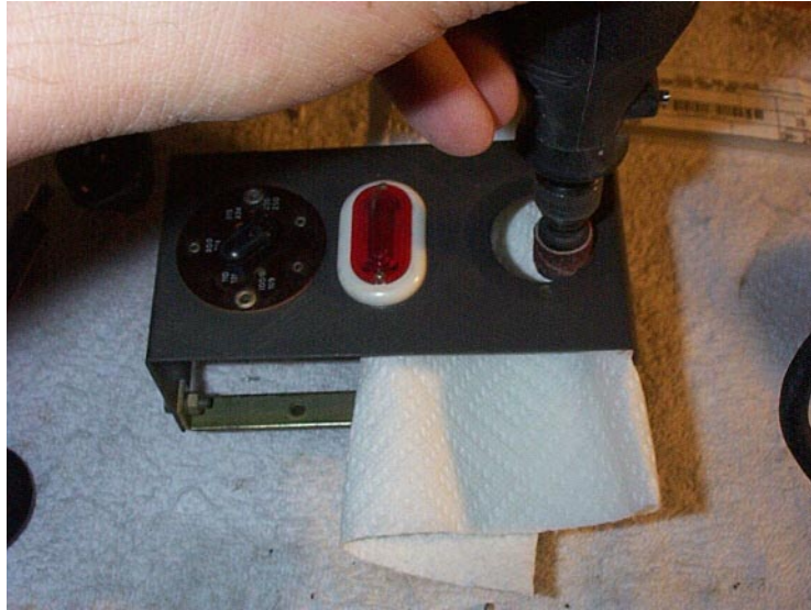
Figure 6.15: Grinding Round Hole For A Square Plug
