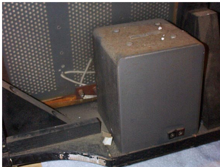
Figure 3.5: ESL Input Transformer Assembly
