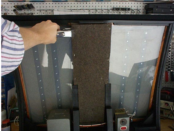
Figure 8.19: Stapling Rear Felt To Treble Panel
