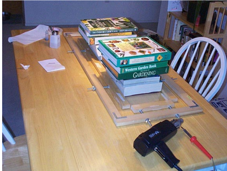
Figure 5.18: Weighting Panel While Epoxy Cures
