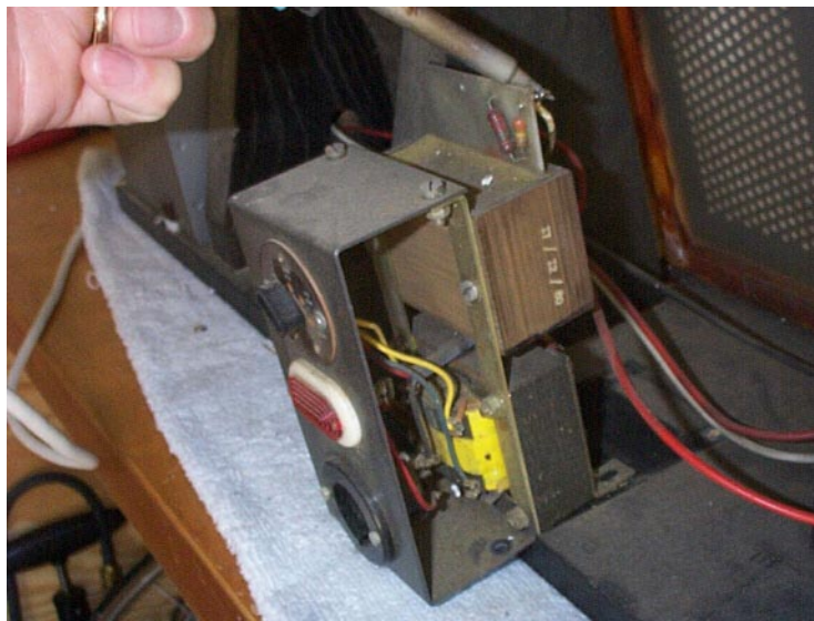
Figure 3.14: Unsolder Power Supply Connections
