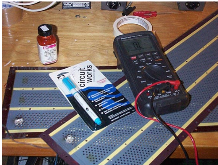
Figure 5.10: Conductive Paint Repair
