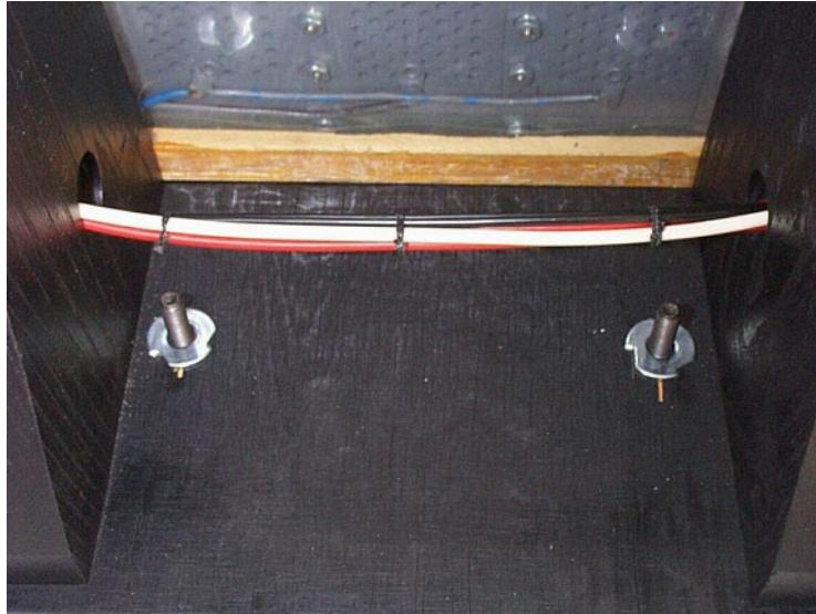
Figure 8.14: Wiring Neatly Dressed and Ready For Final Assembly
