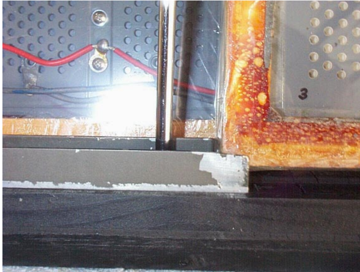
Figure 8.6: Installing the Bottom Retaining Bracket
