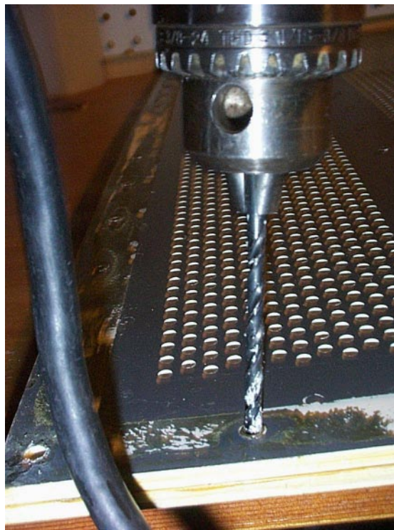
Figure 4.7: Drilling A Bass Panel Rivet
