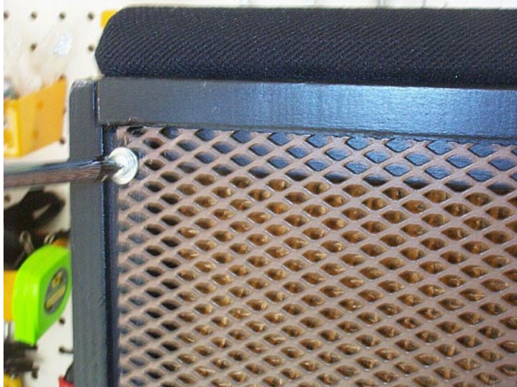
Figure 8.20: Screwing The Rear Grille In Place
