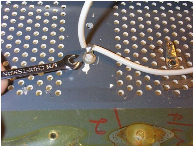
Figure 4.5: Removing The Bass Bias Wiring Harness
