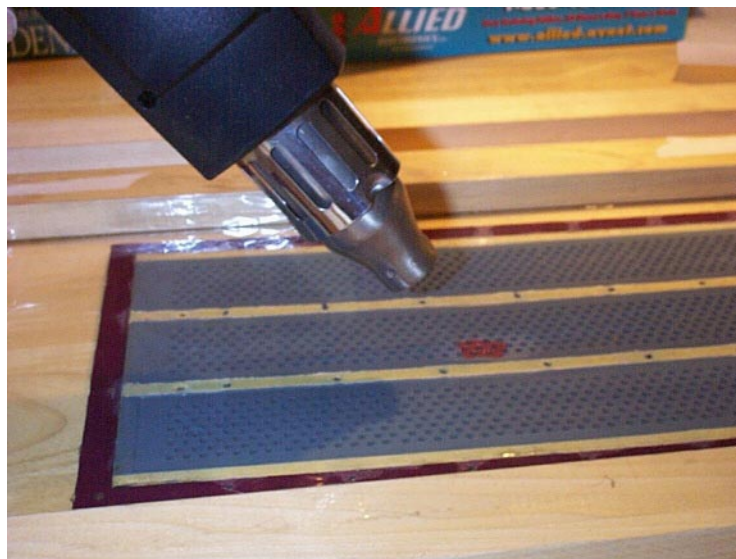
Figure 5.19: Heat Shrinking Treble Panel
