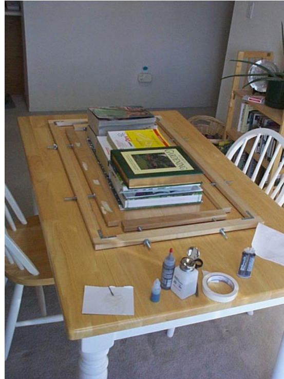
Figure 4.13: Bass Panel Diaphragm Curing
