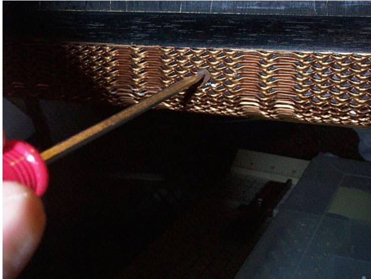
Figure 3.8: Removal of Front Grille Retaining Screws
