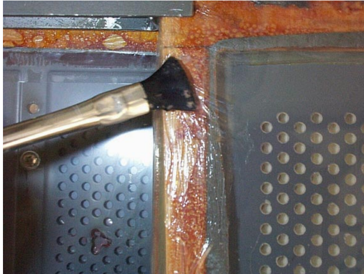
Figure 8.17: Applying Glue For Front Grille Pads
