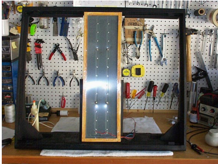
Figure 8.1: Treble Panel Installed In Frame
