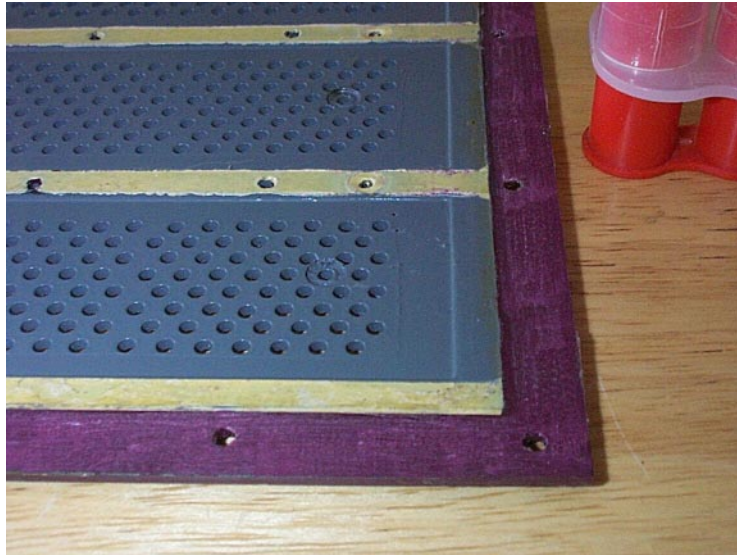
Figure 5.12: Treble Panel With Previous Epoxy Ground Off
