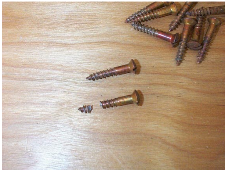
Figure 8.22: Shortening The Side Trim Strip Screws
