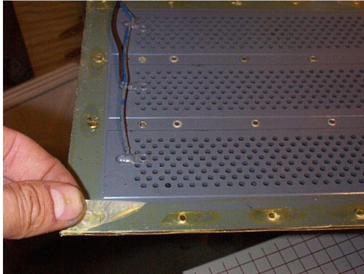
Figure 5.5: Removing The Insulating Tape
