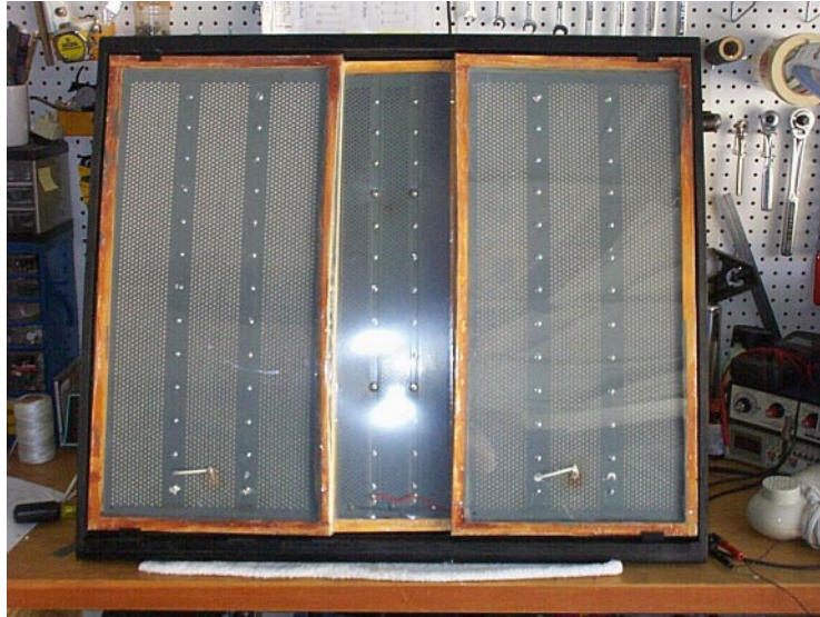
Figure 8.4: Bass Panels Pushed Into Position
