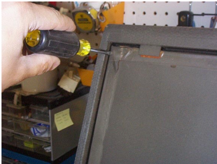
Figure 3.19: Removal of Bass Panel
