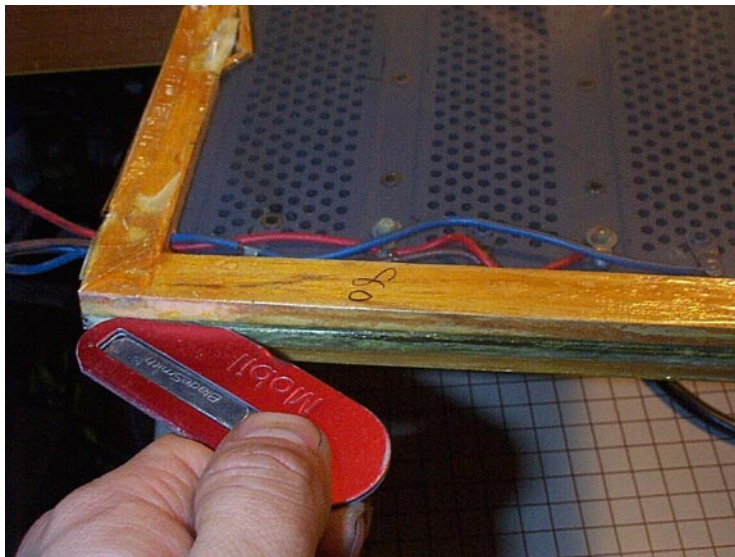
Figure 5.4: Removing The Dust Cover
