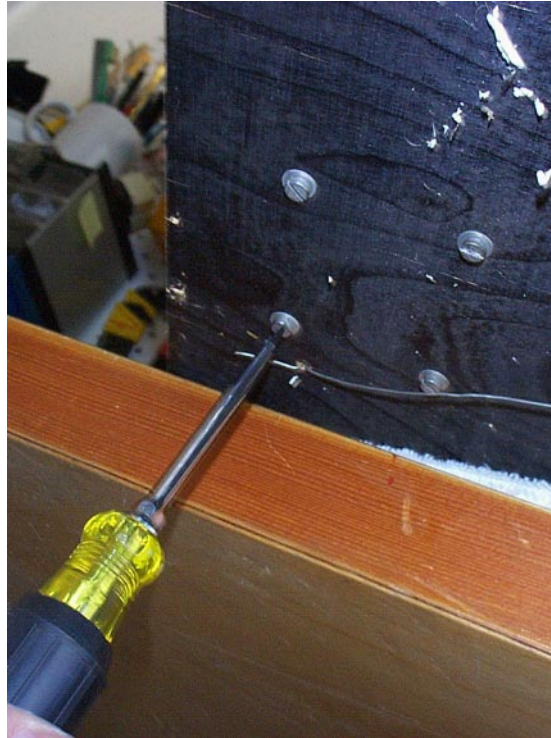
Figure 3.13: Removal of Power Supply Retaining Screws
