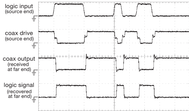
Figure 12.116. Waveforms from a 74AUC1G04 inverter operating at 1.8 V and directly driving a 30 cm length of coax, with the same pulse pattern as earlier, but at a 10 ns clock rate. The four traces (top to bottom) correspond to points A, C, D, and E in Figure 12.114, but with no resistor. The approximate half-step at the coax input confirms a drive impedance close to 50 Ω. Horizontal: 20 ns/div; vertical: 2 V/div.
