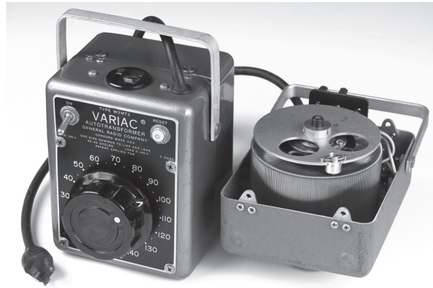
Figure 1.129. A powerline variable transformer ("Variac") lets you adjust the ac input voltage to something you are testing. Here a 5 A unit is shown, both clothed and undressed.
