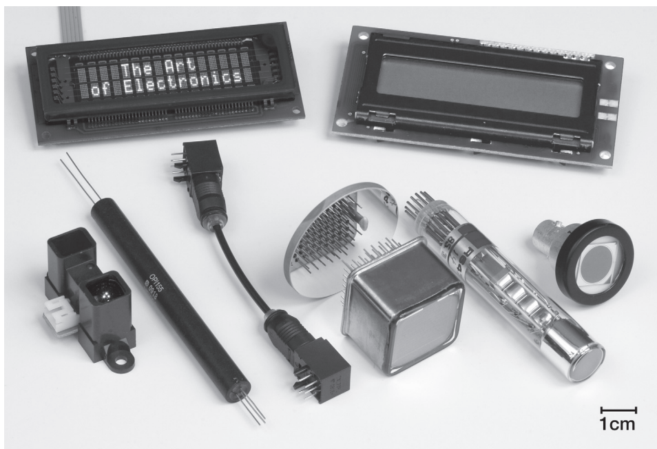
Figure 12.71. A collection of optoelectronic devices too large to fit in Figures 12.58, 12.80, and 12.84. At rear are VFD and LCD smart displays (Newhaven M0216SD-162SDARC-1 and Optrex DMC16207), the former with 3-wire serial interface. In front, left to right, are a ranging/proximity detector (Sharp GP2Y0D02YK0F), a 50 kV logic-output opto-isolator (Optek OPI155), a homemade TOSLINK isolator (Toshiba TOTX/TORX177PL), an 8×8 multianode photomultiplier (Hamamatsu R5900-00-M64), an end-on 13 mm PMT (Hamamatsu R647), and a 10 mm PIN-diode detector (OSI/UDT PIN-10D).
