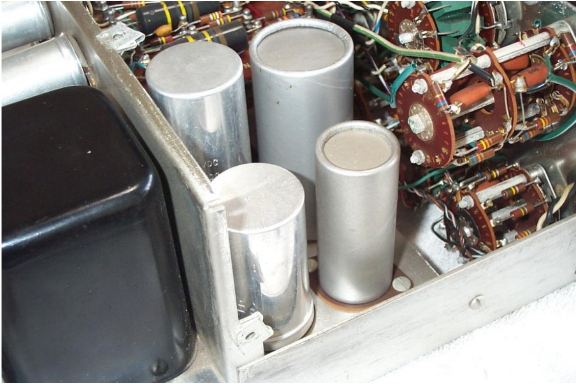
Original Can Capacitors
