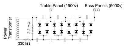
All Diodes: 1N4007 All Capacitors: 0.01  $\mu$ F 2 kV
