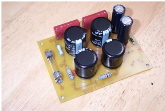
PAS Power Supply Capacitor Board
