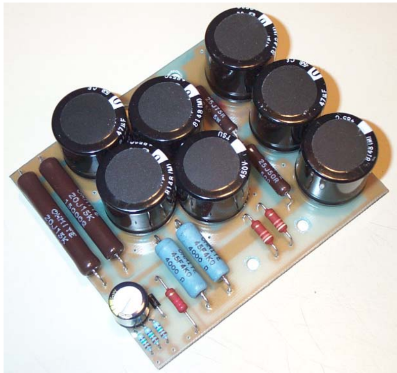
Fisher SA-100 Power Supply Capacitor Board
