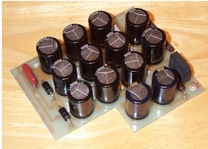
Fisher 500C Power Supply Capacitor Board
