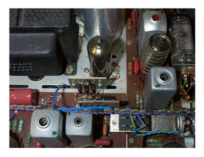
Figure 1: New PEC boards in a Dyna FM3
