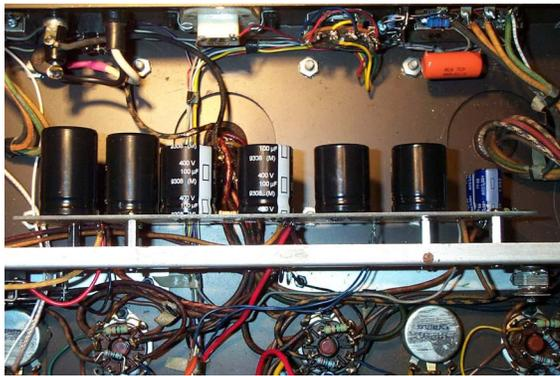
Capacitor Board Installed in Amplifier
