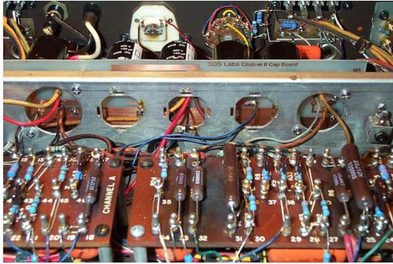
Capacitor Board Installed in Amplifier
