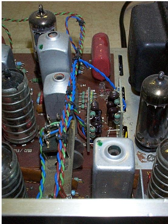
Figure 2: New PEC boards in a Dyna FM3
