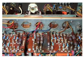
Capacitor Board Installed in Amplifier
