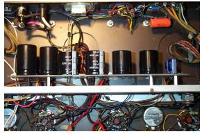
Capacitor Board Installed in Amplifier
