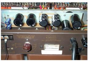
Capacitor Board Installed in Amplifier
